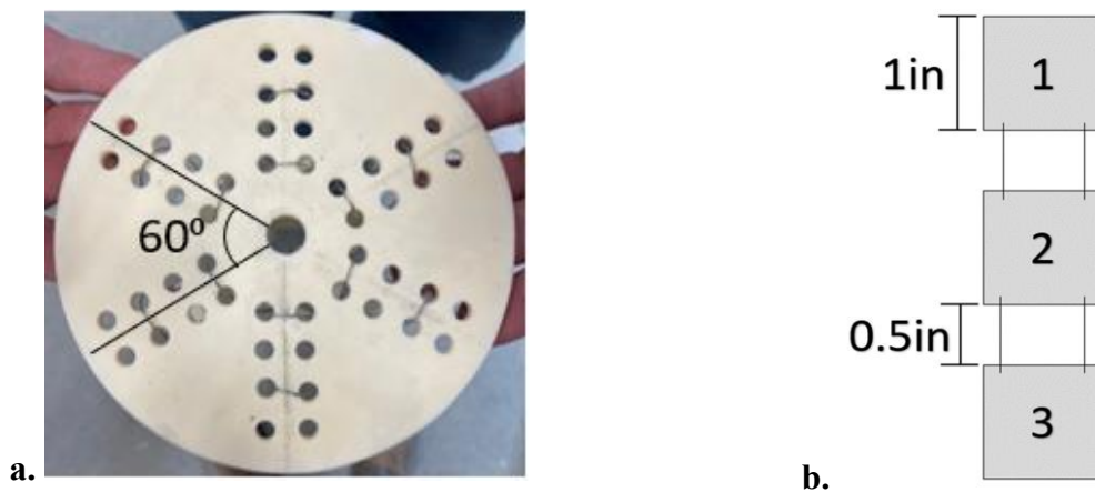
FIGURE 2. (a) Alumina Disk Machined to hold Samples, and (b) Display of how samples were hung
