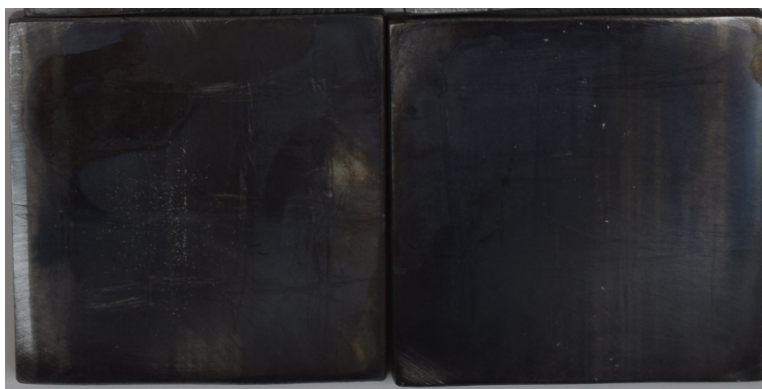
Figure 4: Dark blue surface oxide that forms on 303 and 416 stainless steel surfaces from citric acid passivation. Formation of the dark layer occurs during the passivation process itself. Incorporation of an alkaline pre and post treatment resulted in the elimination of the discoloration, and surfaces that appeared similar to that illustrated in Figure 1B.
