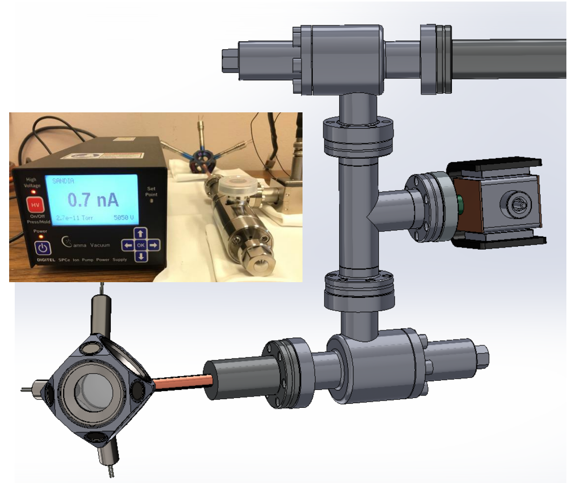
Solid-model of Titanium chamber/UHV manifold assembly
