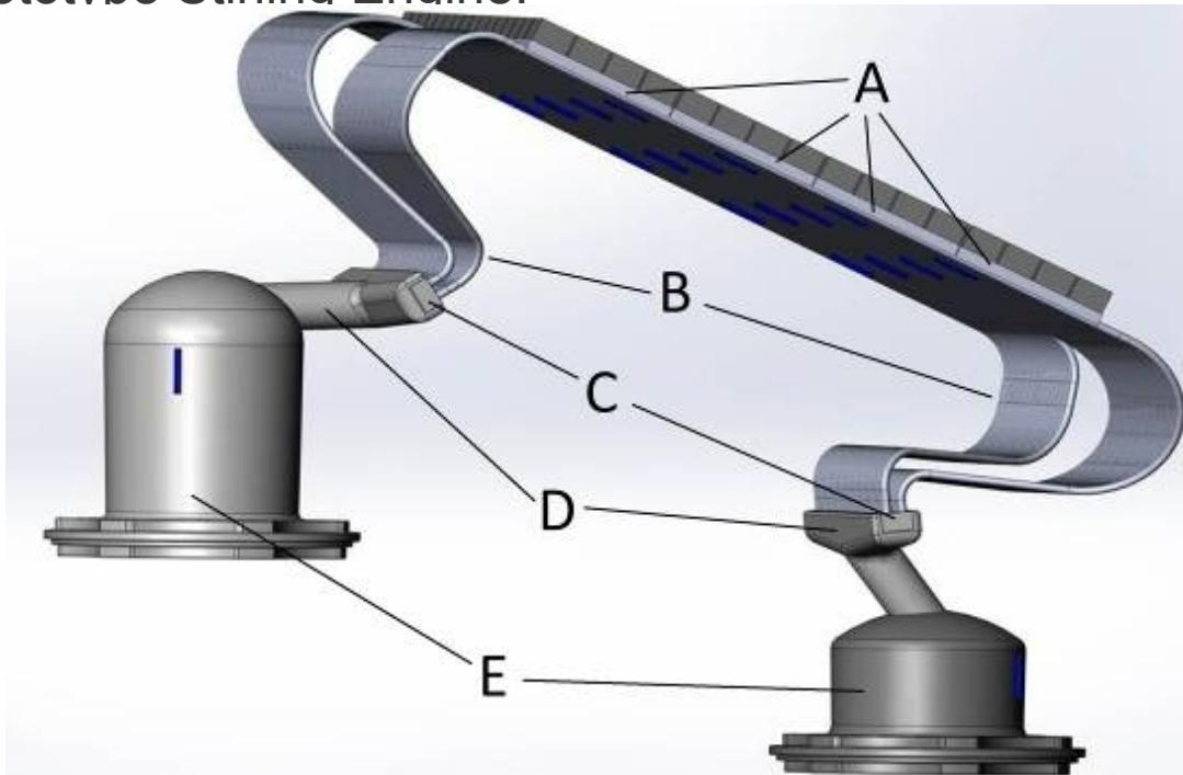
A computer rendering of a Stirling Engine heat exchanger. Components are:
