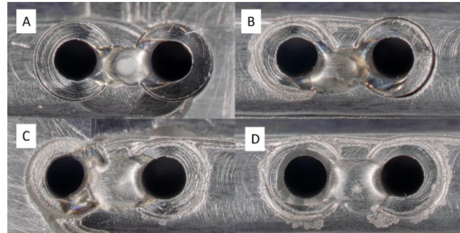
The 0.125" (3.175mm) gas tubes are set flush to the inside surface of the Header and TIG welded prior to brazing. The depth setting shims (TIG welded to the center divider) are removed prior to brazing
