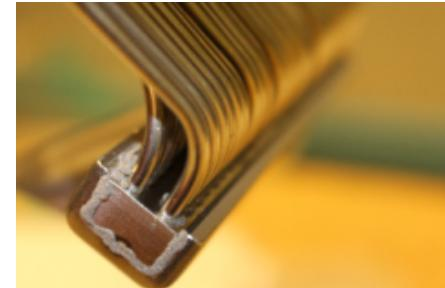
The Gas Passage Tubes are aligned lengthwise by clamping the ends between two Alumina rods. The EM Tile Array plane is fixtured by clamping tubes down to a Kovar setting plate with Alumina plates in between and Alumina strips separating the tubes from each other. More Alumina plates and SS304 weights are placed on top of tubes during brazing run.
