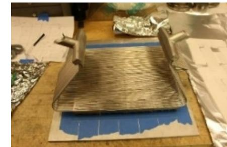
Assembly is lifted-clamped-then inverted for transfer to furnace raised platform (molybdenum bars, Kovar cylinders, Alumina shims) Note: Alumina shims between ALL adjacent tile faces.
