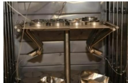
The Gas Passage Assembly is leak tested following the braze cycle using a Varian QualyTest Helium Mass Spectrometer. Because the system is designed to contain Hydrogen at high temperatures and pressures there is no acceptable leak rate. No leaks are detected.
