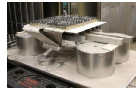
Assembly is centered between furnace hotzone sides/elements & partially inserted into hotzone. SS304 Cylinders 6lbs (2.7kg) are placed atop each tile. Entire arrangement fully inserted into furnace.
