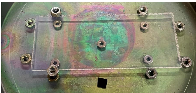
Figure 7. Picture of full-sized ( \sim 15.5 \times 7 \times 0.4 \text{ cm} ) tile in ALD chamber. Nuts are used to prop up the tile and facilitate diffusion of precursor to the bottom side of the tile.
