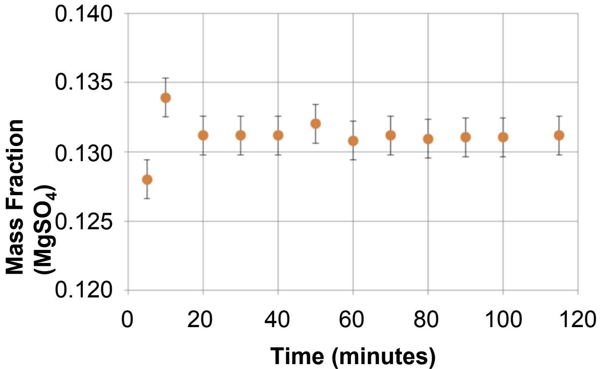
Salt (surrogate) concentration was determined by measuring the ionic conductivity of the neutralent. Most of the salt was extracted from the debris within 30 minutes. Testing showed that  $8.2 \pm 4\%$  of the salt remained occluded in the plastic bags.
