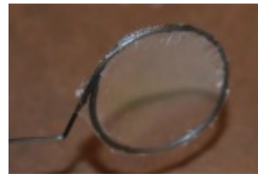
FIG. 4. Photograph of the Mylar window. The nominal thickness from the manufacturer is 1 \mu\text{m} . However, 850 nm thickness is found to better agree with the measurement. This discrepancy may be due to either the thickness or the uncertainty in the X-ray attenuation factors at low energy. 5
