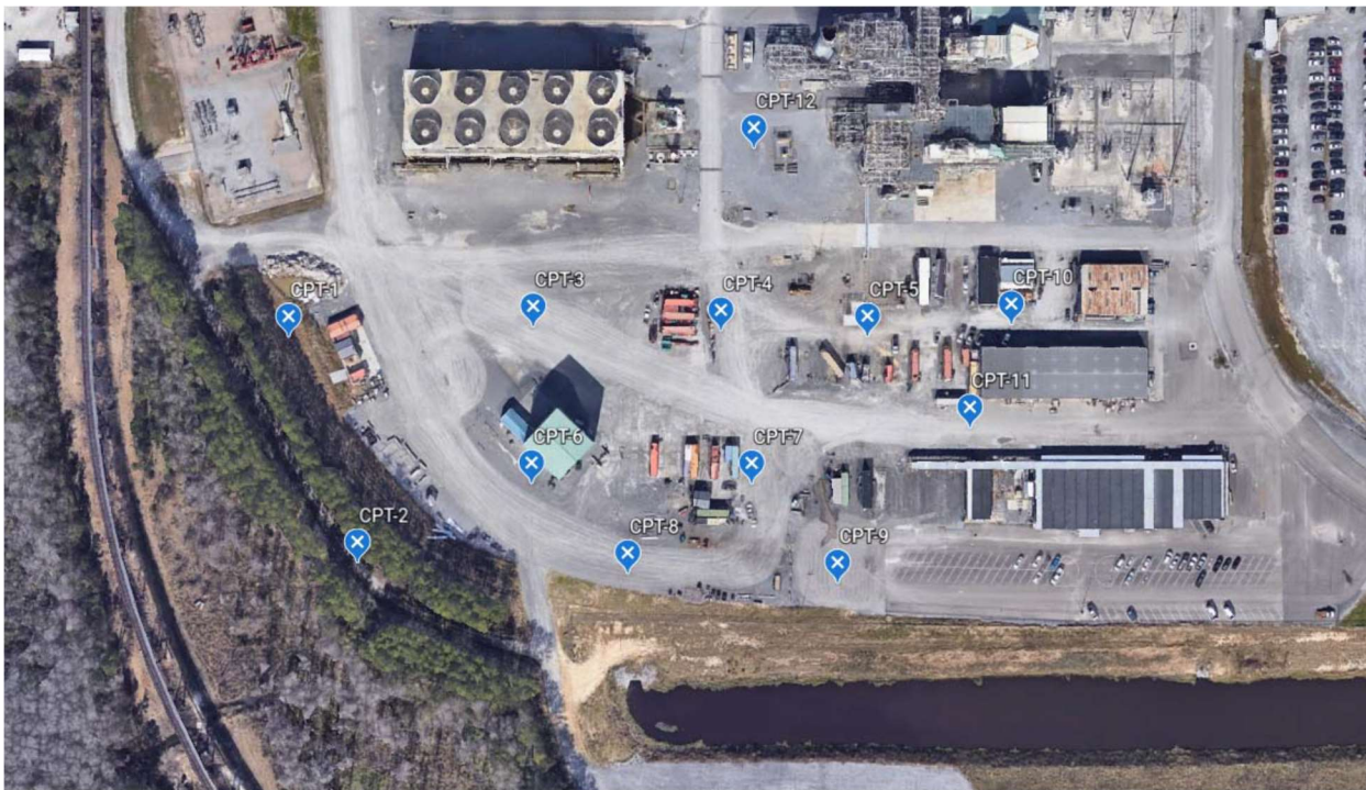
Figure 2: Cone Penetration Test Plan for Plant Daniel
