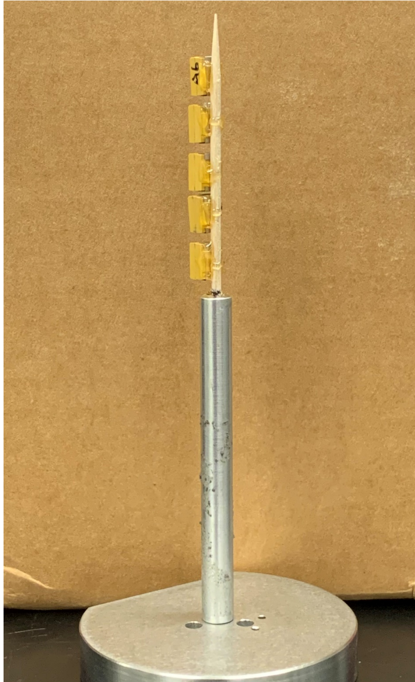
Figure 1 – Five Ta capacitors mounted to toothpick and Al rod
