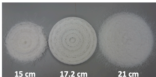
Figure 7. Three different sizes of extruded and cured sorbents. The goal is to cut the sorbents to a certain size dry, then hydrate them to ~40% to obtain a final 20.3 cm in diameter.
