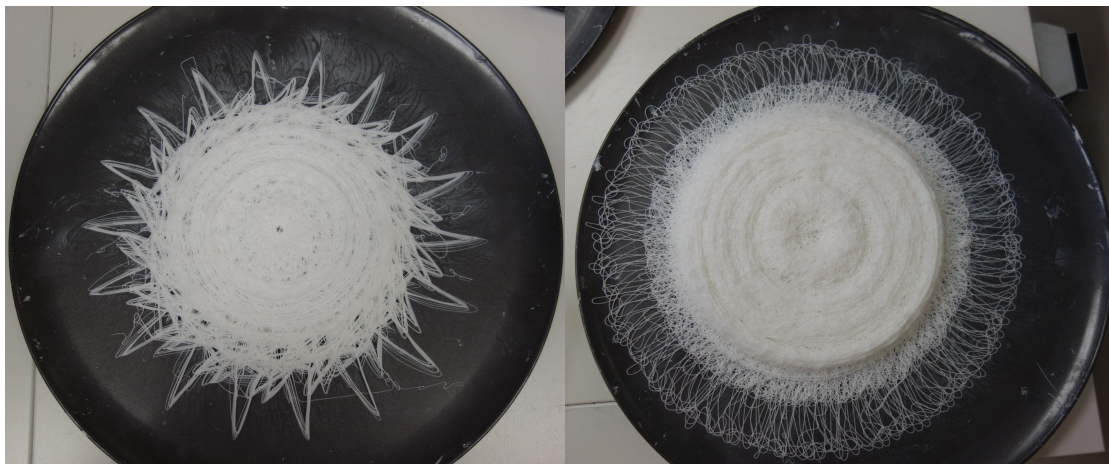
Figure 12. Finished printed and cured patterns of composite sorbents using different nozzle positions. Different nozzle positions have a significant effect on how the pattern will look in the end. The height of the composite sorbent depends on how many cycles are run.
