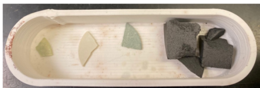
Figure 16: Sample color changes after annealing \text{ZrW}_2\text{O}_8 , \text{HfW}_2\text{O}_8 and \text{HfMgW}_3\text{O}_{12} in \text{N}_2 at 700 °C and 1100 °C.
