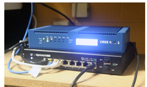
Lighting network POE switch and Link server.
