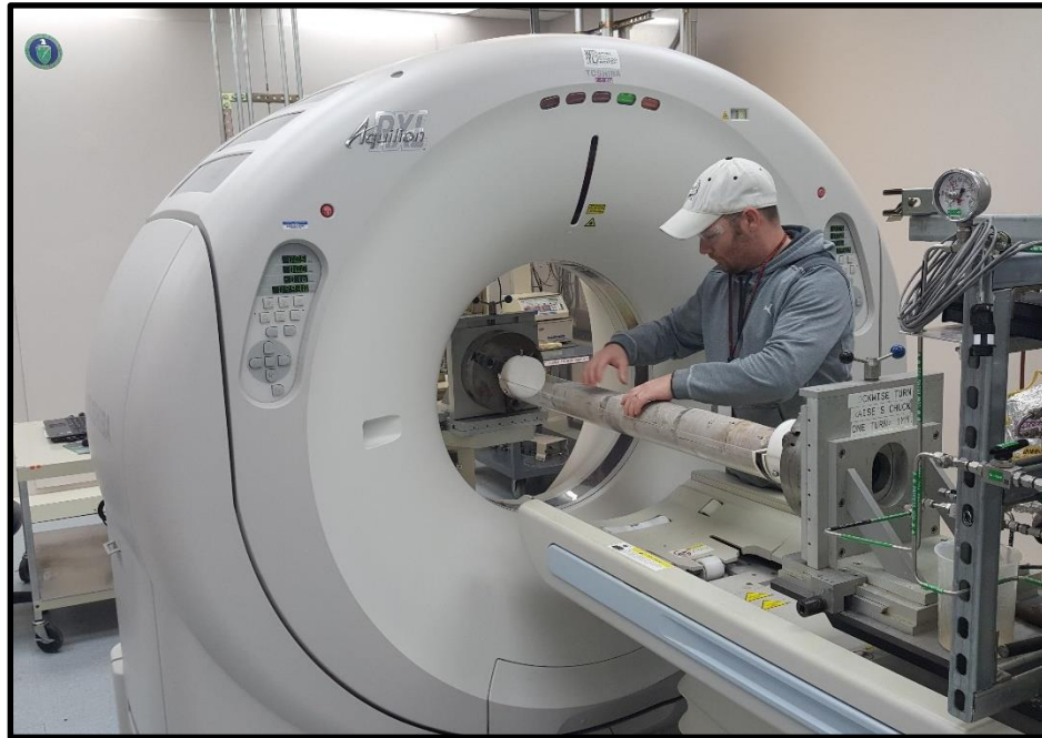
Figure 4: Toshiba® Aquilion™ Multislice Helical CT Scanner at the NETL used for core analysis.
