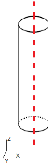
Figure 10: Schematic of the XZ isolated plane through the vertical center of the medical CT scans.
