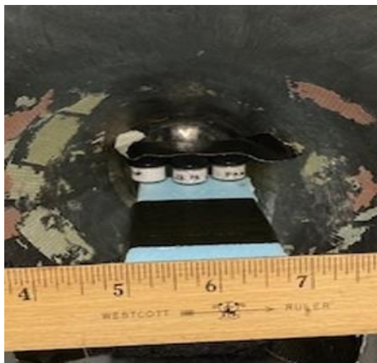
Figure 9. SBMOF-1 composites secured in Co-60 gamma-ray beam port.
