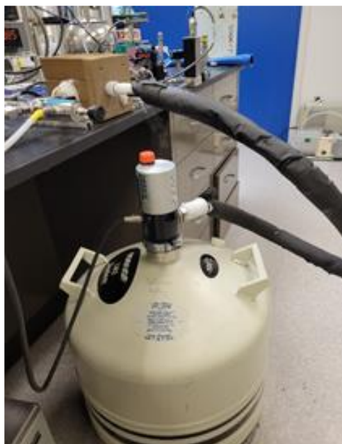
Figure 14. Micro-dosing liquid nitrogen system
