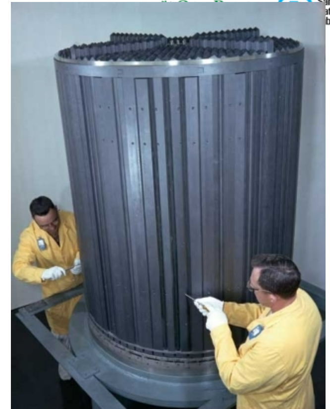
MSRE Graphite Core Structure [ https://en.wikipedia.org/wiki/Molten-Salt_Reactor_Experiment ]
