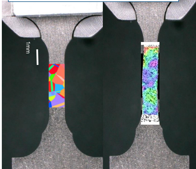
Specimen with pre-test EBSD and post-test DIC overlays
