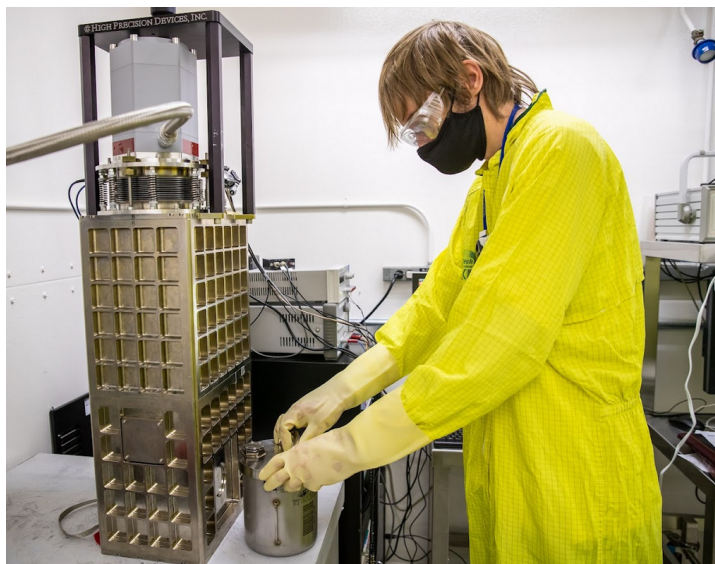
Figure 3: Items to be measured were placed next to the detector window on the side of the cryostat. Typical packaging consisted of SAVY containers.
