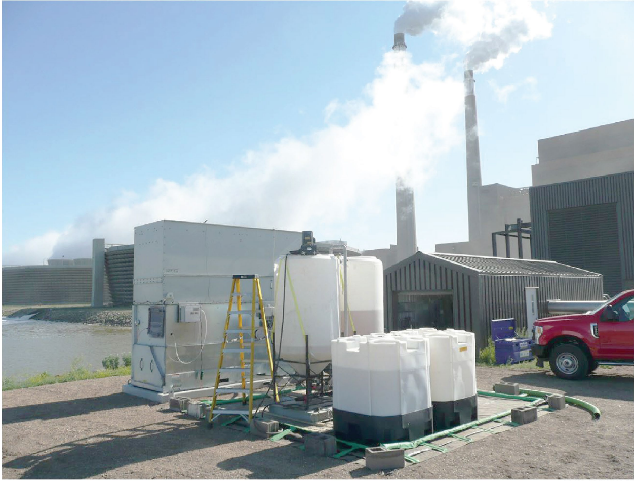
Figure 6. Pilot hygroscopic cooling system installed at Coal Creek Station.
