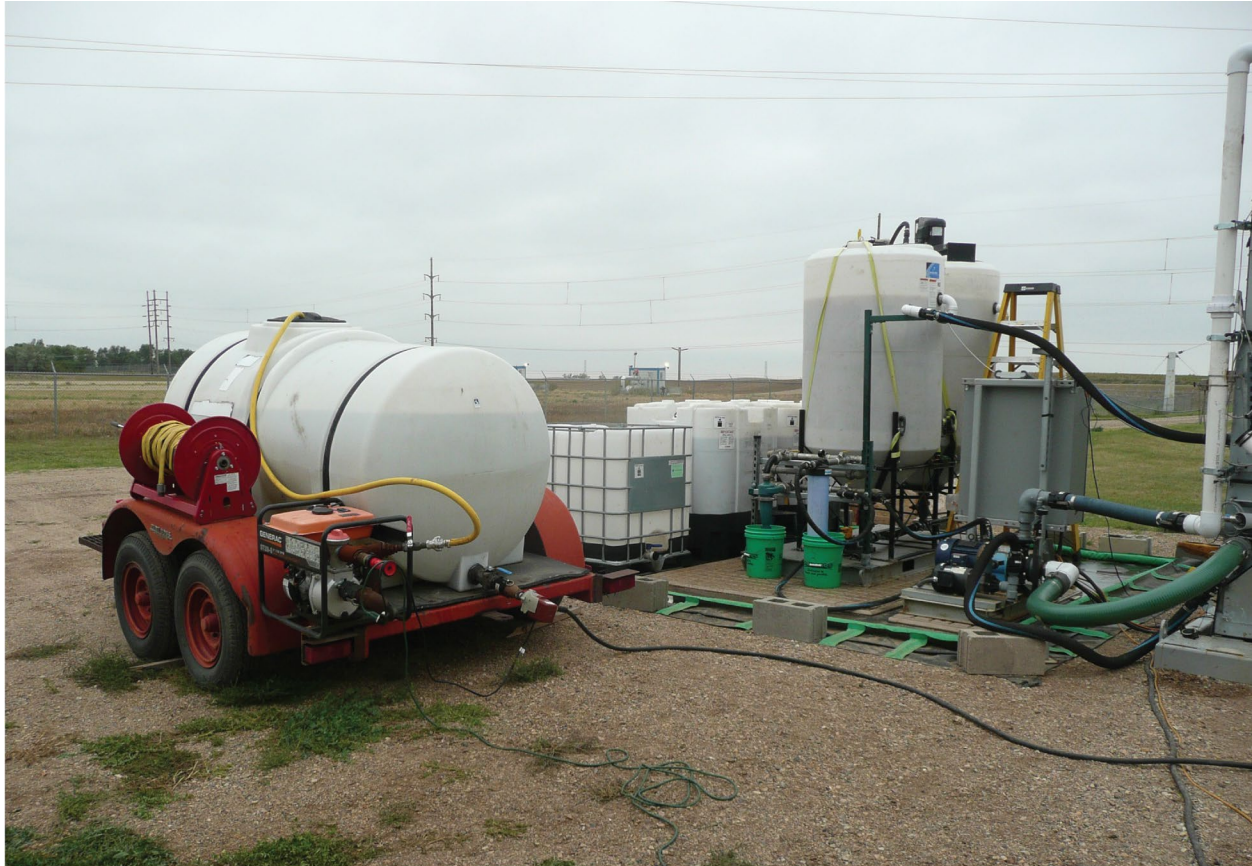
Figure 9. Portable tank, at left, used to bring APW to the test unit.
