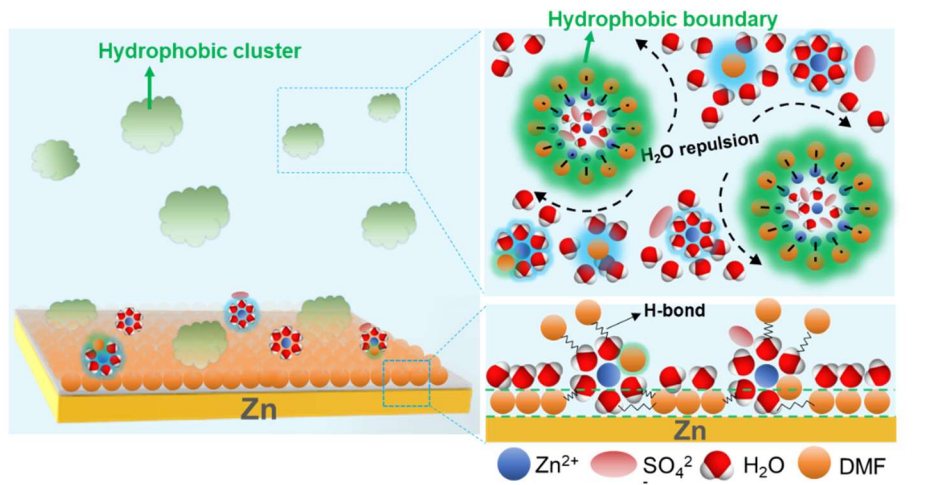
Localized hydrophobicity and interfacial alkalinity-scavenging in \text{ZnSO}_4\text{-H}_2\text{O-DMF} electrolyte
