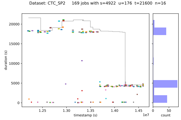
Fig. 1. Predictor behavior for an example job group with a multimodal distribution. Job start time is on the x -axis and run time is on the y -axis. Boxes are individual jobs and the grey line is the predicted run time. The histogram on the right shows the frequency of jobs with a particular run time.
