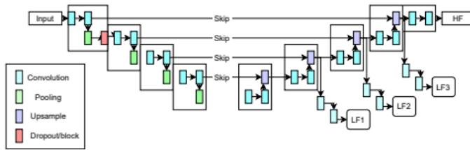
Next, we will investigate generalizations using combinations of low or high dimensional inputs/outputs using composable encoder-decoder architectures.
