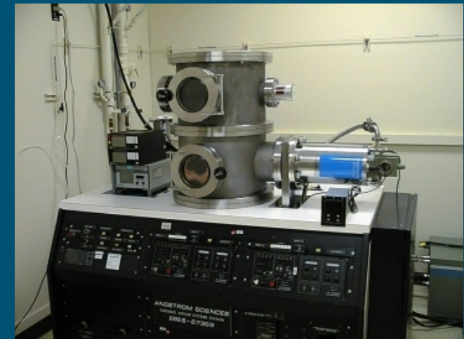
Dual e-beam evaporator located at Sandia Nation Laboratories
