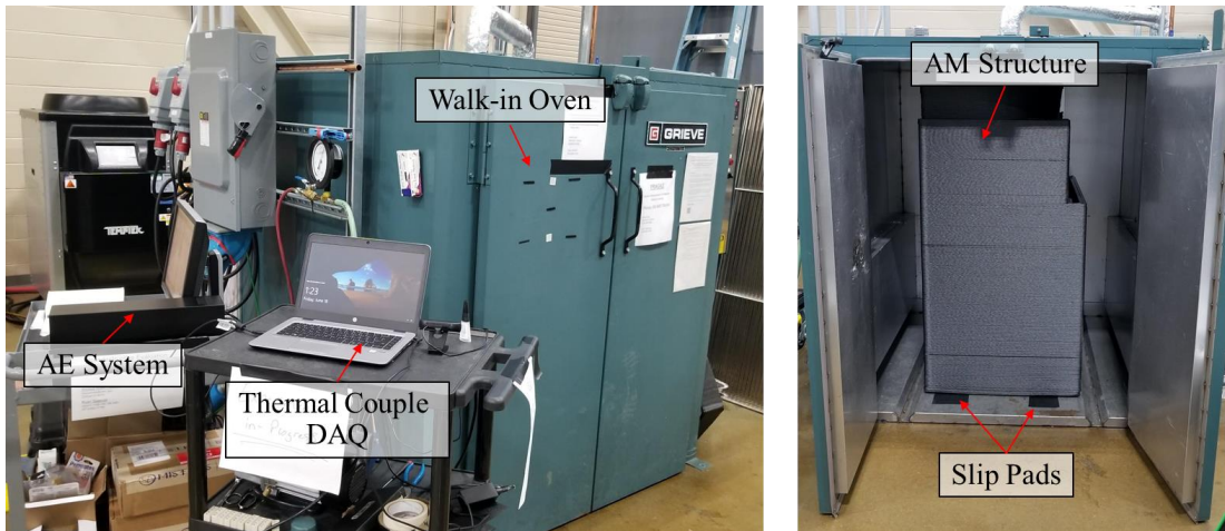
Figure 2: Thermal cycle setup with GRIEVE walk-in oven, thermocouple DAQ system, and the AE system. The AM Structure was placed on smooth slip pads to allow thermal expansion and reduce frictional noise.
