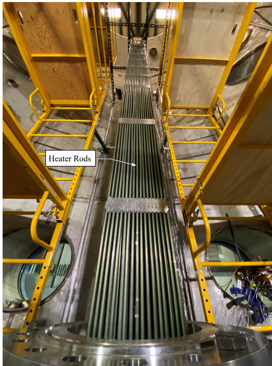
Figure 2-4 PWR skeleton fully outfitted with waterproof heaters.
