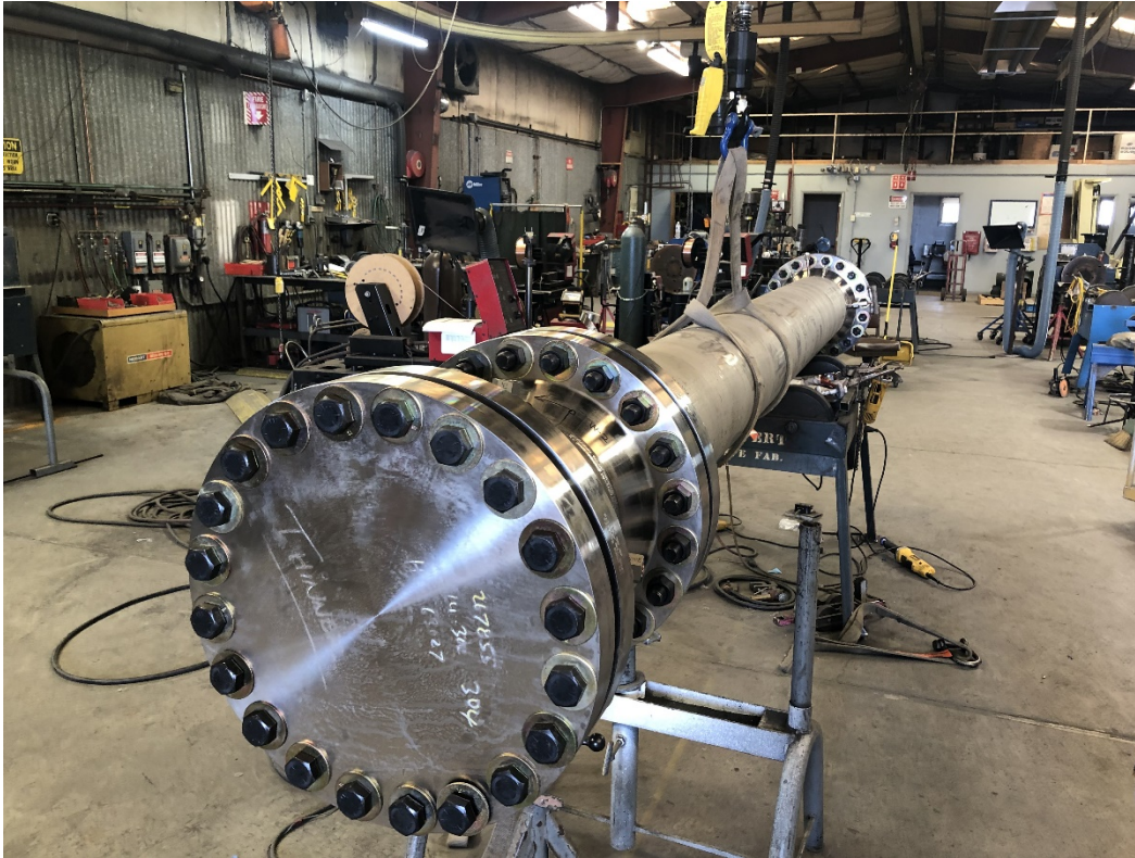
Figure 2-9 Photo of the ADCS pressure vessel taken during hydrostatic testing. The ADCS vessel is divided into lower and upper pressure vessels.
