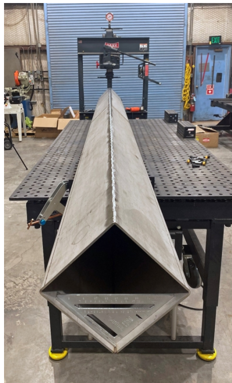
Figure 2-6 Completion of basket fabrication through application of machine press to maintain 90-degree corners on basket interior.
