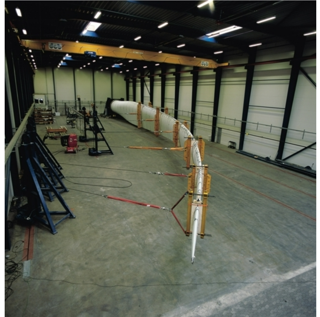
Blade under high deflection during structural testing
