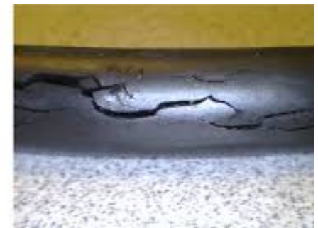
Damage in polymer O-Rings after hydrogen gas exposure
