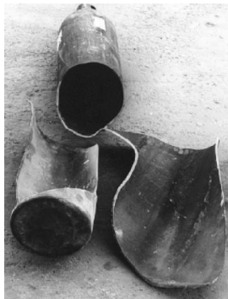
Rupture of hydrogen-containing metal tanks
