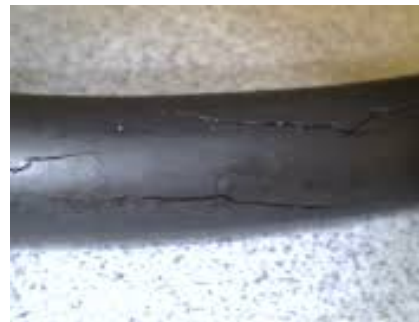
Damage in polymer O-Rings after hydrogen gas exposure
