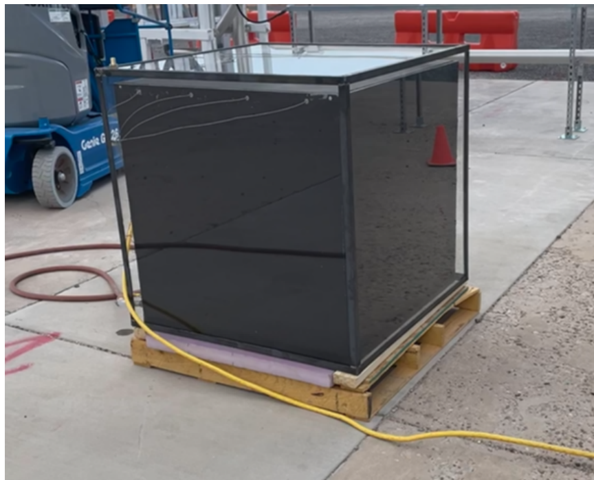
Figure 2-6. Fully-instrumented glaze solar collector placed outside the assembly building to enable solar heat collection.
