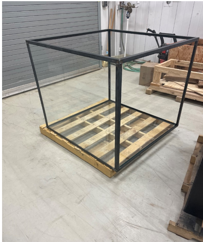
Figure 2-2. Glaze structure showing the glass and support iron rods.
