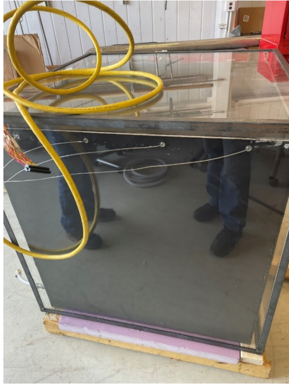
Figure 2-5. Instrumentation of the glaze, fractal-fin solar collector assembly.
