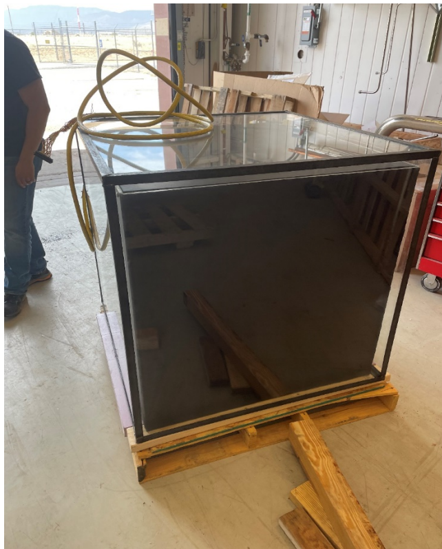
Figure 2-4. Fractal-fin solar collector inside the glaze containment.
