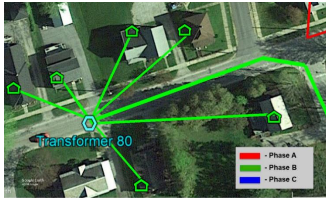
Figure 4-28. Phase labels as predicted by the phase identification algorithm and verified in Google Street View for a transformer on Utility #2, Feeder #3
