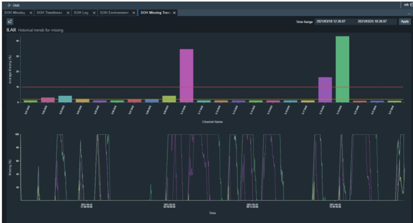
In this view of the SOH Missing Trends Display, the Average Missing data percentage is shown for each channel for the Time Range selected. The lower panel shows a trend plot for each channel, with colors matching the upper display. The channels shown may be down-selected to reduce complexity.
