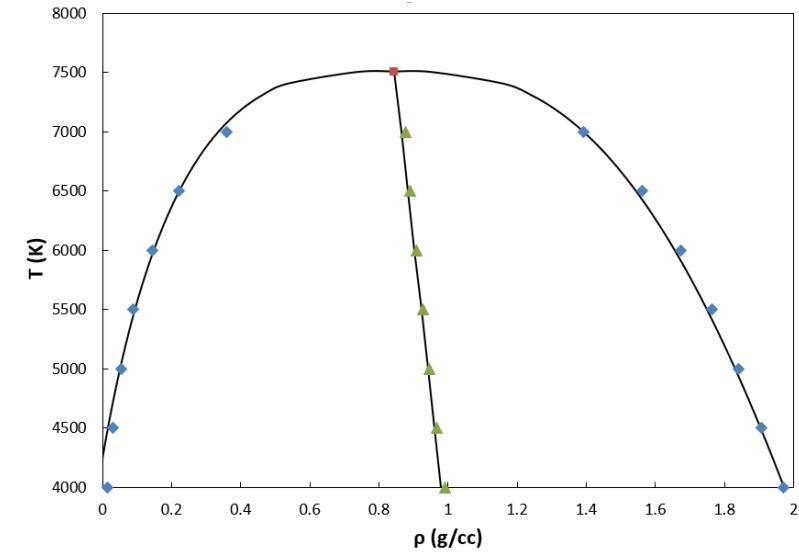
*Take Home Message: The physically realistic SNAP machine-learning potential captures liquid-vapor coexistence behavior for free expansion of aluminum at a level not generally accessible to hydrocodes.*
