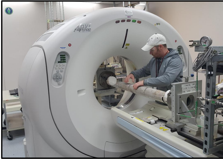
Figure 17: Toshiba® Aquilion™ Multislice Helical CT scanner at NETL used for core analysis.
