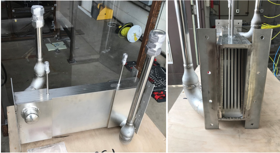
Figure 4-1 Photos of the 20 kW t heat exchanger core after manufacturing at VPE and prior to testing at Sandia
