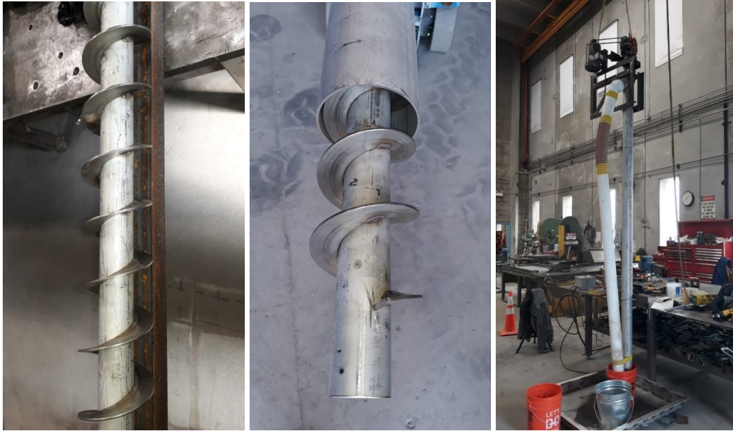
Figure 2-7 Photos of the screw lift assembly and low-temperature commissioning setup
