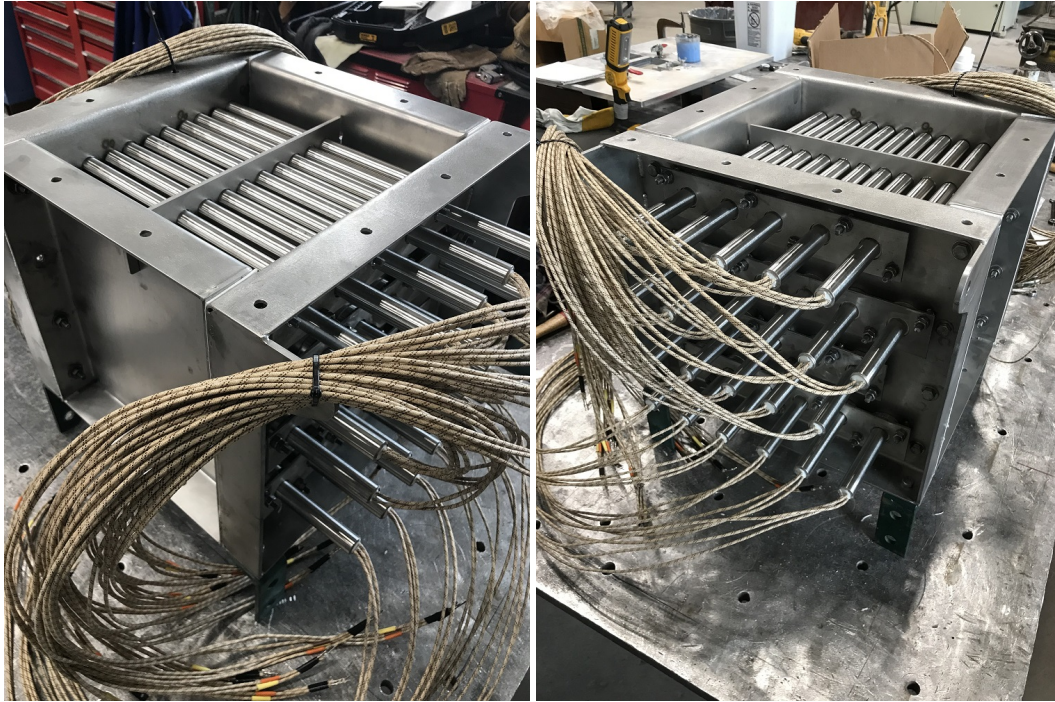
Figure 2-5 Image of the assembled 60 kW t particle heater prior to installation in the heat exchanger test stand
