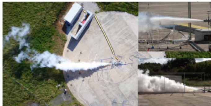
Figure 3-18. Visible cloud during dispersion and rainout tests at HSE facility.
