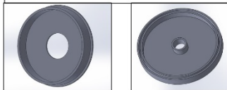
Discs to hold Boron Carbide & Concrete Mold
