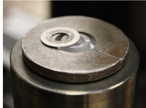
Fractured sample, still in tensile grips.
