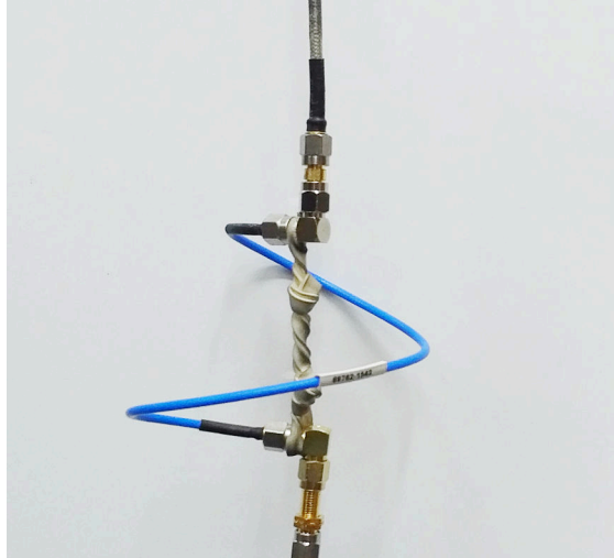
Figure 4-3. Flexible cable link connection used to allow vessel rotation while maintaining high isolation.
