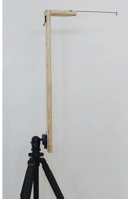
Figure 4-2. Wood holder used for near-field probe placement.
