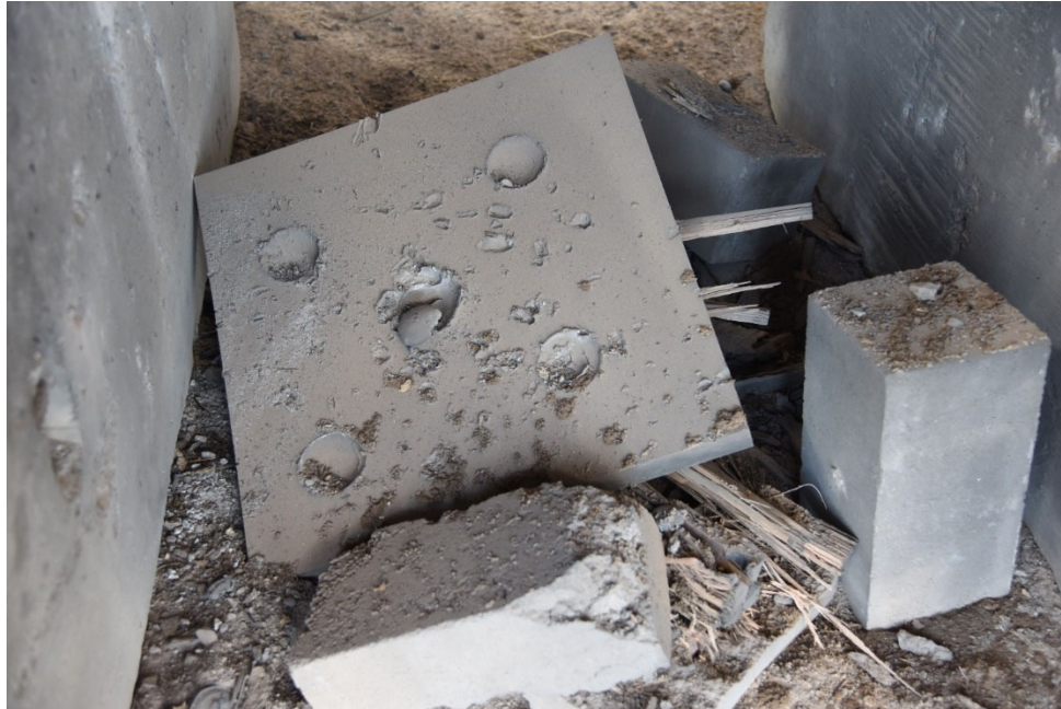
Figure 18. Aluminum Target Plate Resting Position Post-Flyer impact
