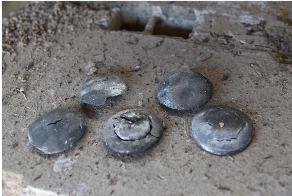
Figure 19. Five Flyer Plate Remnants Post-Target Impact
