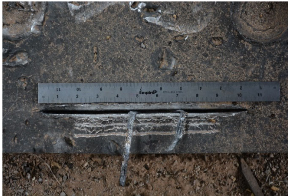
Groove Created in Aluminum Target
