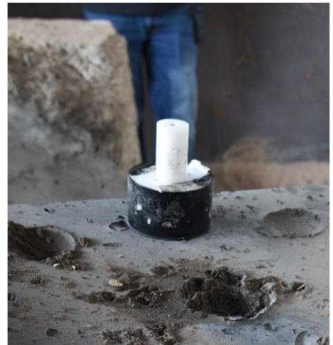
Figure 7. Experimental 0.75 in. Copper Conical Shape Charge
