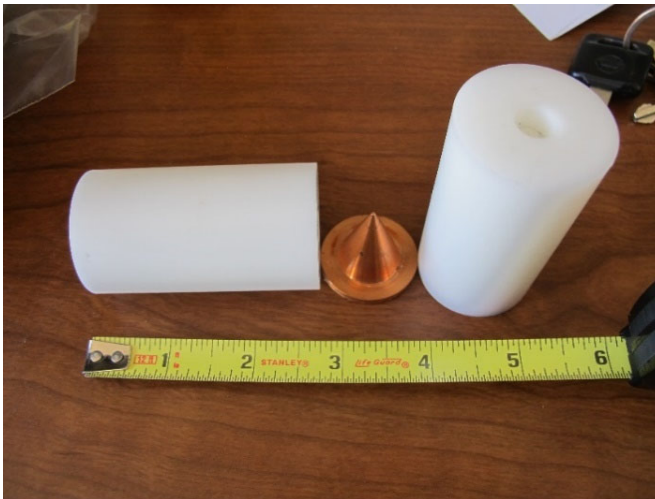
Figure 7. Experimental 0.75 in. Copper Conical Shape Charge
