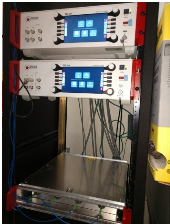
Toptica laser system for 369 nm, 399 nm, 760 nm, & 935 nm
