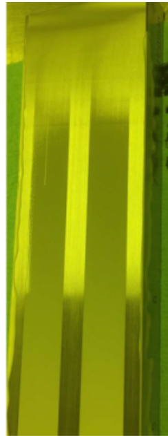
Typical Fineness of Grind gage patterns (from ASTM D 1210-05)
