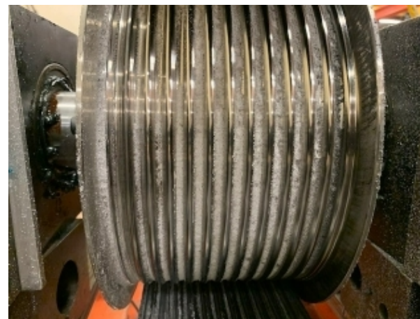
Belt wear debris in drum grooves at 847,612 machine cycles.
