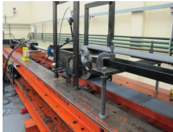
Tensioning drum clevis assembly attached to load cell and hydraulic tensioning cylinder
