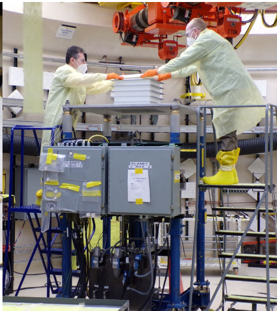
▲ Upper stack of TEX-TSL poly configuration with LANL He-3 detectors and RTD's
