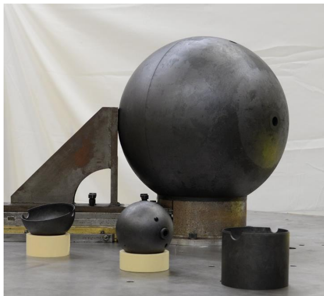
Figure 2. Close-up of Flattop, in Closed Position, with Fullcap, HEU Core, and Pedestal Adapter (L-R) Arranged on the Tabletop.
