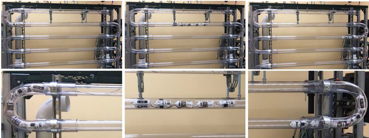
Figure 16 - Crawler navigating the superheater tube mock-up with magnified images.
