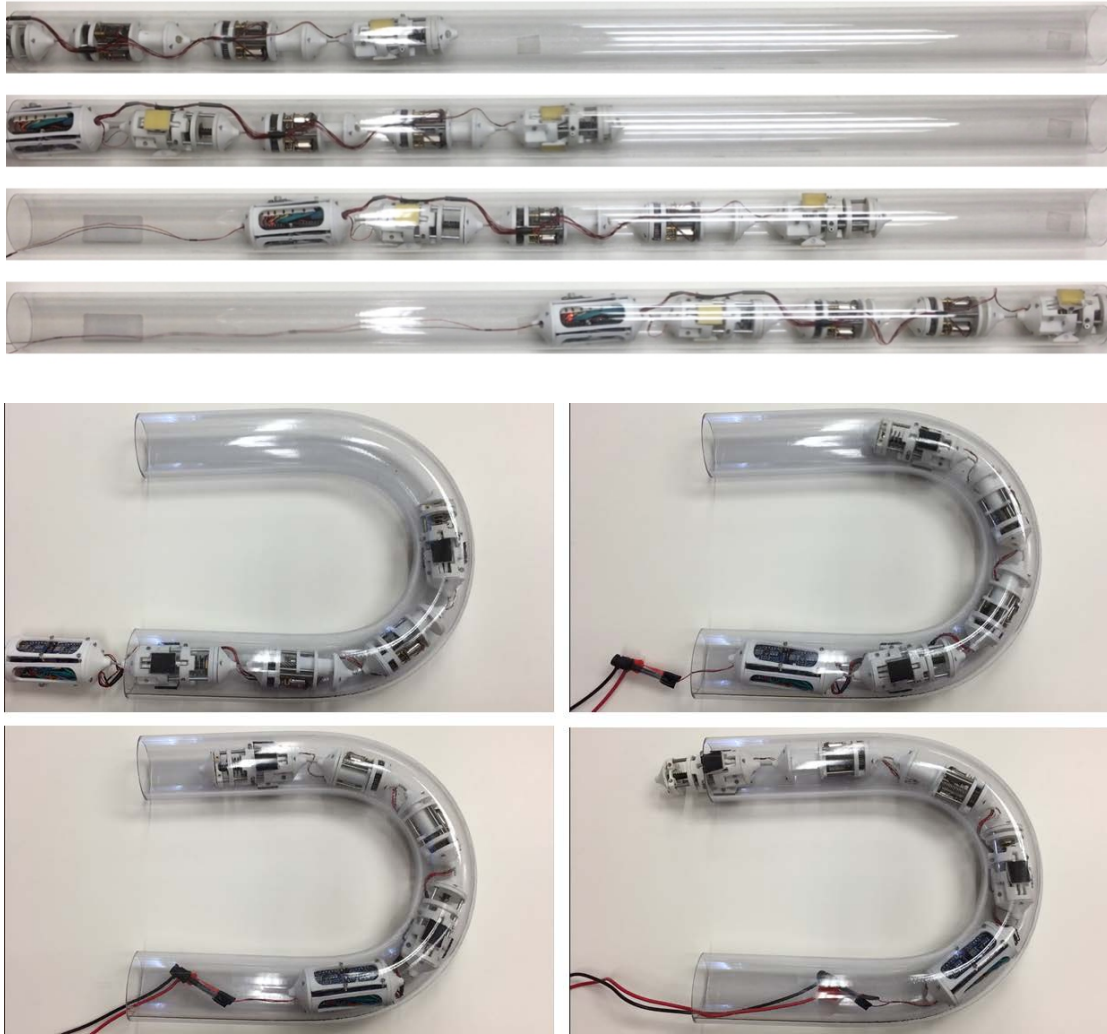
Figure 13 - Robotic crawler traveling in straight tube section and plastic U-bend.
