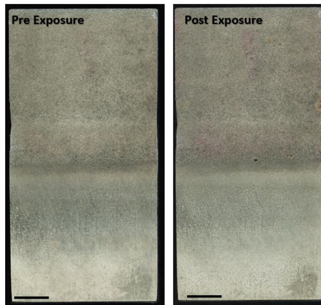
Figure 18: Pre and post exposures for Super C-nitrogen tapered exposed to 75% RH and 35 °C. Scale bars are 5 mm. Cold spray is oriented towards the top of the image, substrate towards the bottom.
