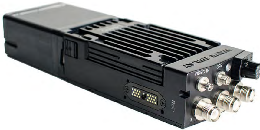
Figure 2. MPU5 radio manufactured by Persistent Systems.
