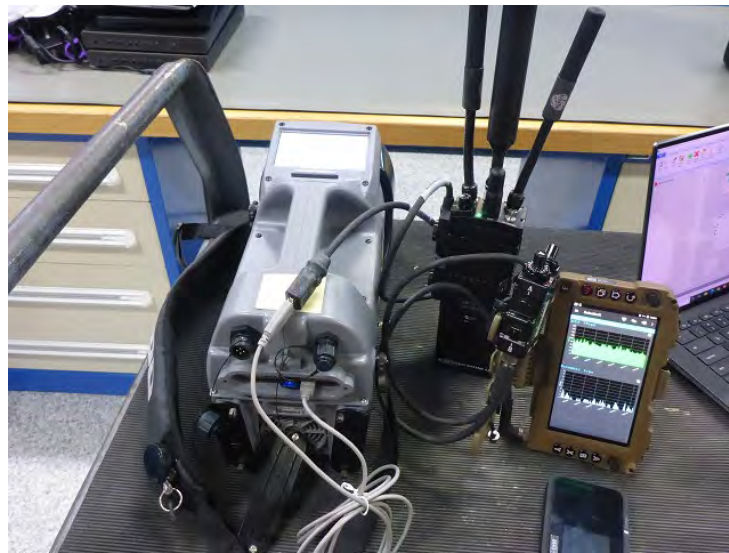
Figure 8. An HPGe radioisotope identification device is coupled with an MPU5 radio to transmit high-resolution gamma energy spectral data to AVID.
