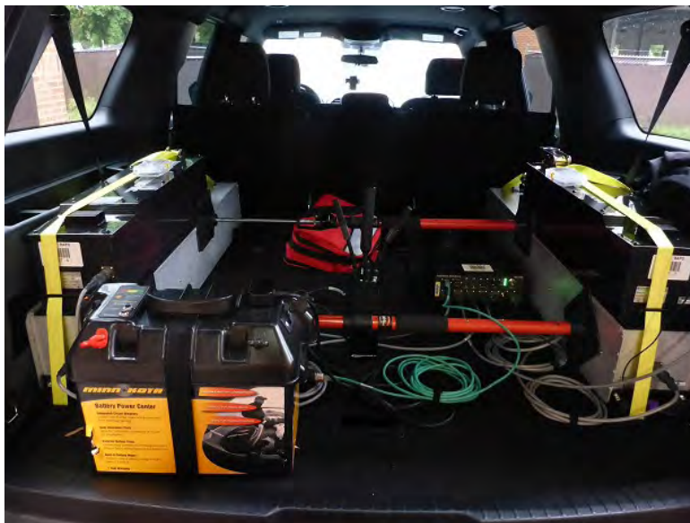
Figure 5. Vehicle-mounted system with two smaller modules of Radiation Solutions Inc. detection system RSX-1. The MPU5 is located in the middle of the picture. The data obtained from the system via AVID is shown in Figure 6.
