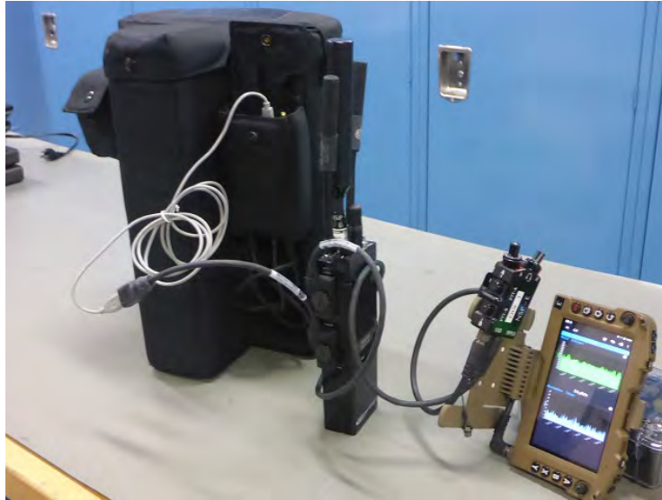
Figure 3. A backpack system set up to transmit radiation monitoring data to AVID by using MPU5 radio. The data received from two such systems is shown in Figure 4, with one of the backpacks causing radiation alarm.
