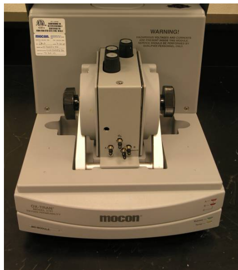
New more sensitive MOCON Ox-Tran 2/21 permeation system
