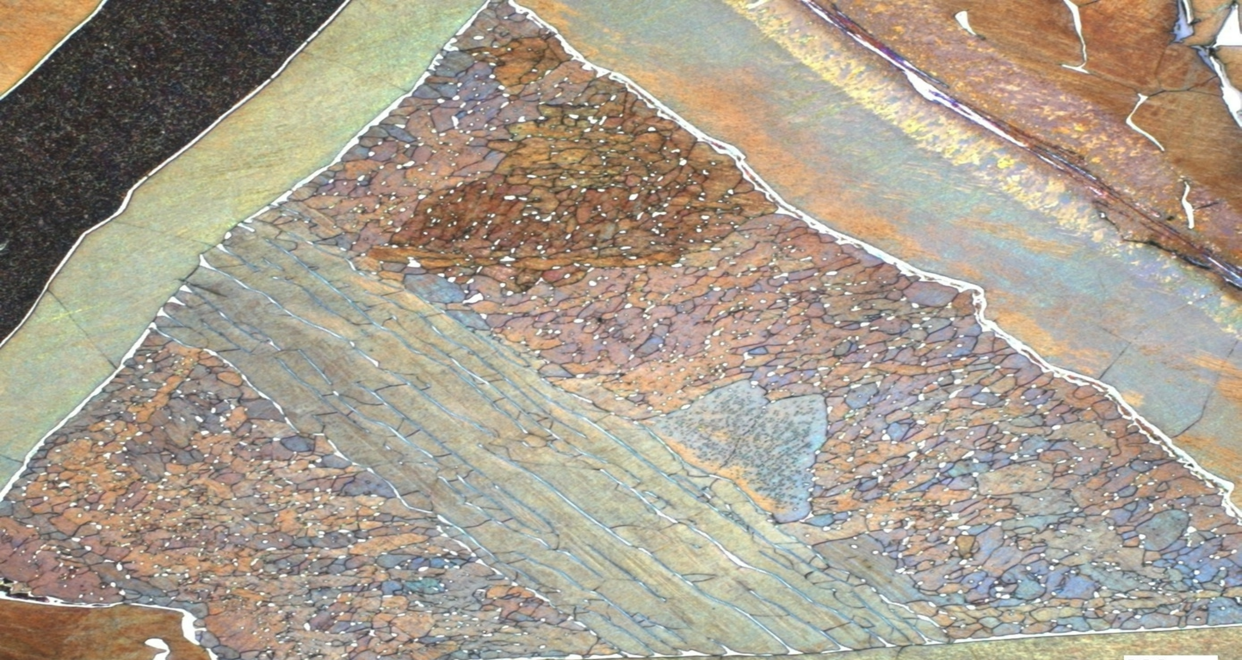
10% Sodium Metabisulfite, 20 seconds, polarized light
