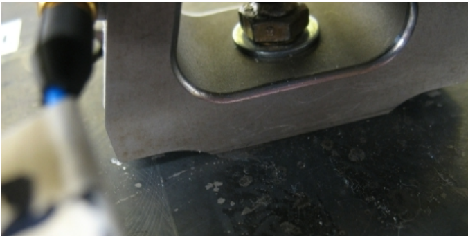
Fig 6. Close-up of contact between the kettlebell and plate
