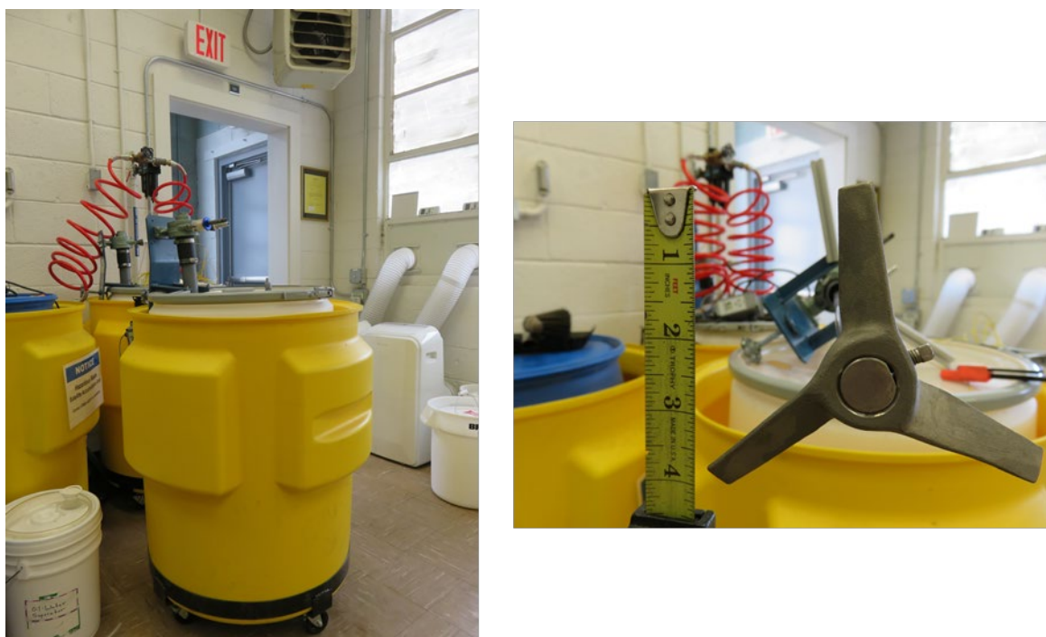
Figure 3: 55-gallon barrel experimental setups with 4 in. axial impeller installed.
