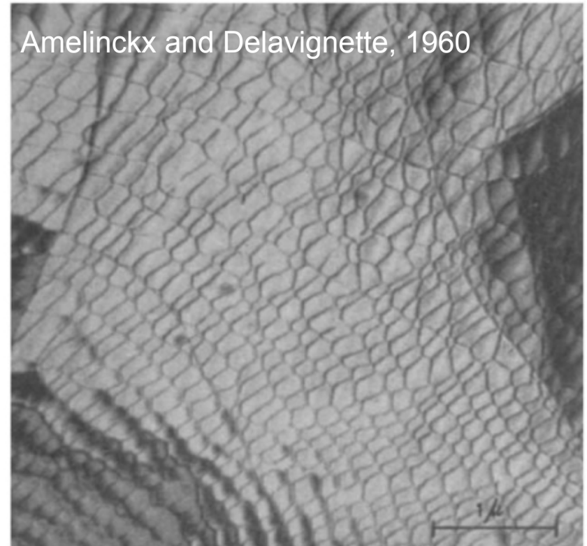
Fig. 1. Dislocation network in Bi 2 Te 3 . Note that certain segments of dislocations and certain node-points have left the foil
